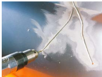
Drilling ends of cracks to relieve stress in the part
