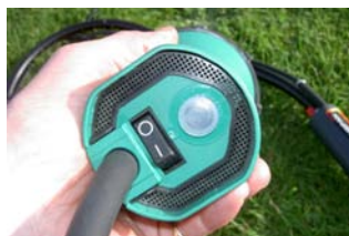
Photo: Rear end of the Soron blower . Wiring connection allow integration of the welding tool.
